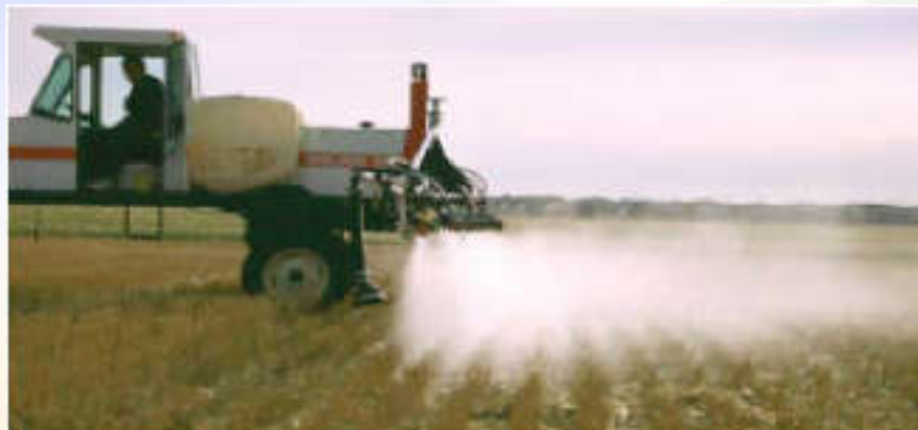
Figure 2. Conventional flat fan spray tips at 40 psi. (Wolf)
