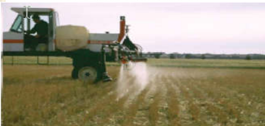
Figure 3. Air induction nozzles at 70 psi. (Wolf)
